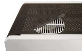
Cutaway above shows the dual high-suction fans located under the 12" wide perforated belt. The fans pull media down onto the conveyor at high speed for optimal transport.
